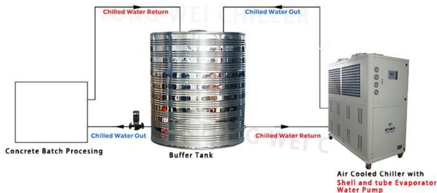
Air-cooled Cement Cooling Chiller Installation Drawing
