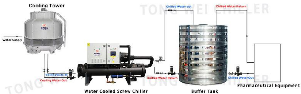
Water-Cooled Pharmaceutical Chiller installation
